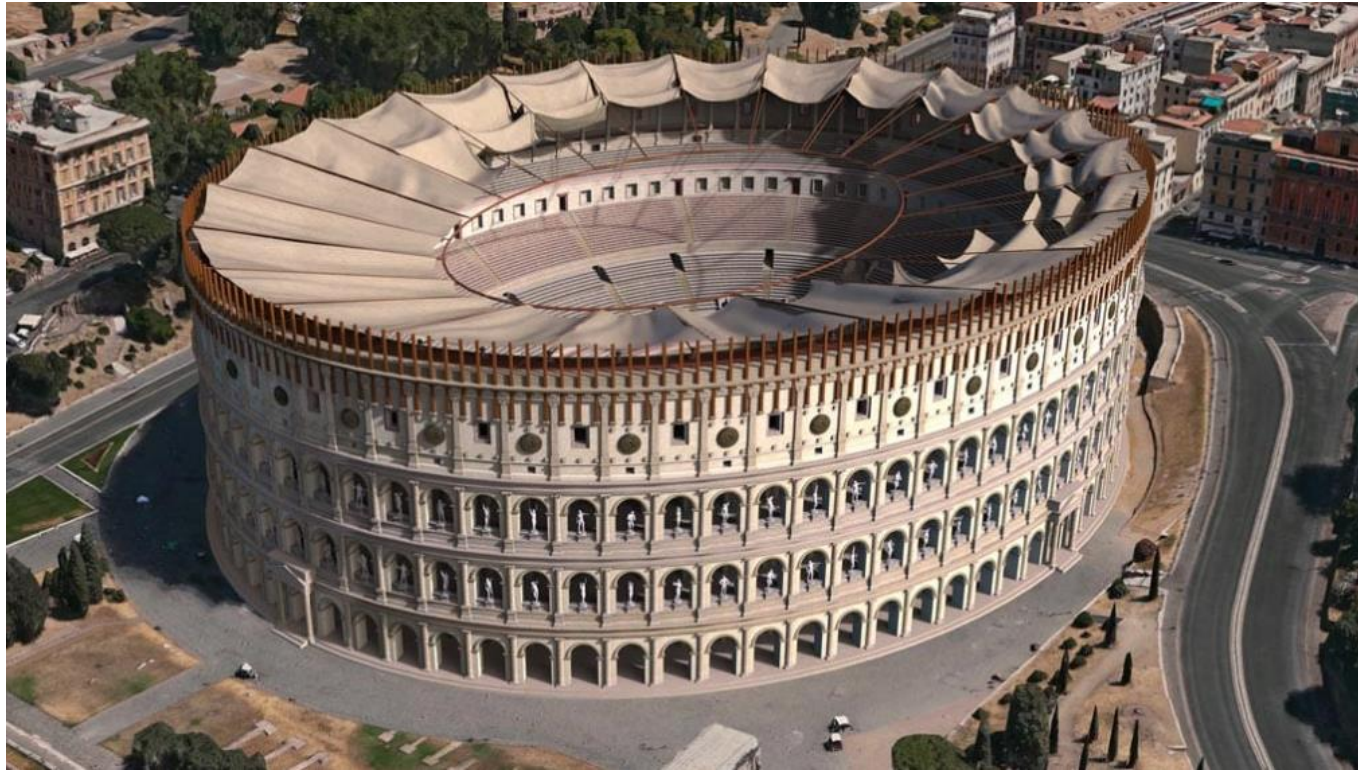
Theorized 3D reconstruction with retractable sailcloth awning (velarium)
