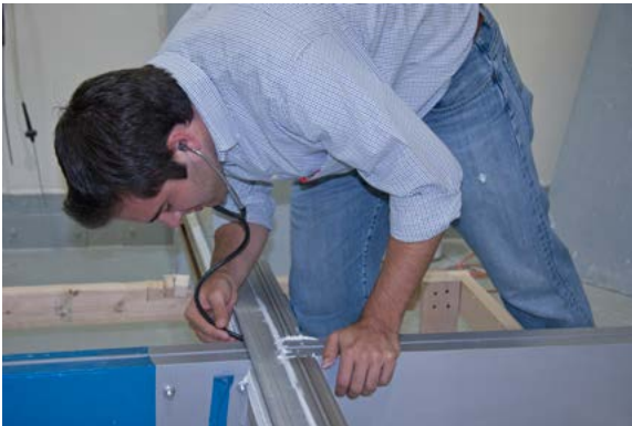
ACOUSTICAL TESTING HAS EXPANDED TO INCLUDE AUDITORY TRANSFER BETWEEN FRAMING SYSTEMS IN CURTAINWALL.
